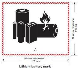
The mark shall be in the form of a rectangle with hatched edging. The dimensions shall be a minimum of 120 mm wide x 110 mm high and the minimum width of the hatching shall be 5 mm. The symbol (group of batteries, one damaged and emitting flame, above the UN number for lithium ion or lithium metal batteries or cells) shall be black on white. The hatching shall be red.
